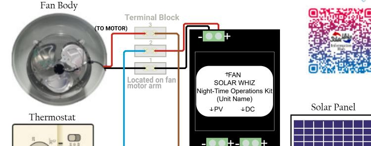
Remove RED WIRE that originally connects terminal 2 and 3 and replace with thermostat as shown in diagram
