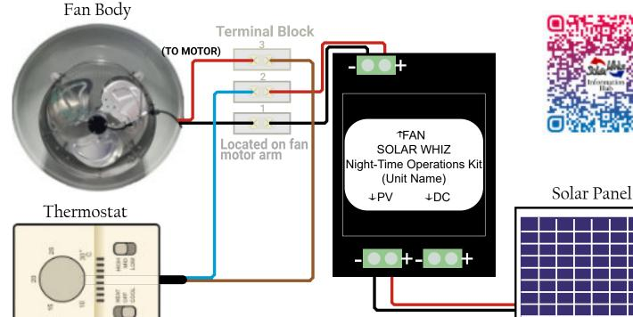
Remove RED WIRE that originally connects terminal 2 and 3 and replace with thermostat as shown in diagram
