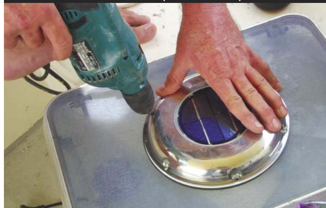
With the vent in place drill holes for the screws.
