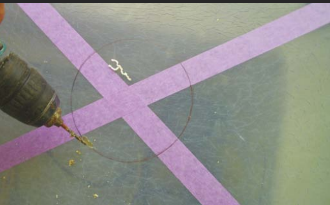
Drill about three holes on the marked circle as a starting point for the jigsaw.
