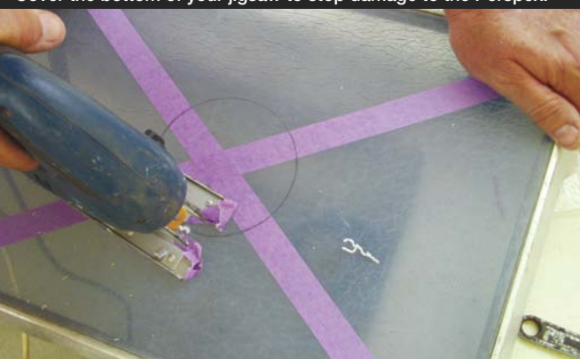
Using a Jigsaw cut out the circle.
